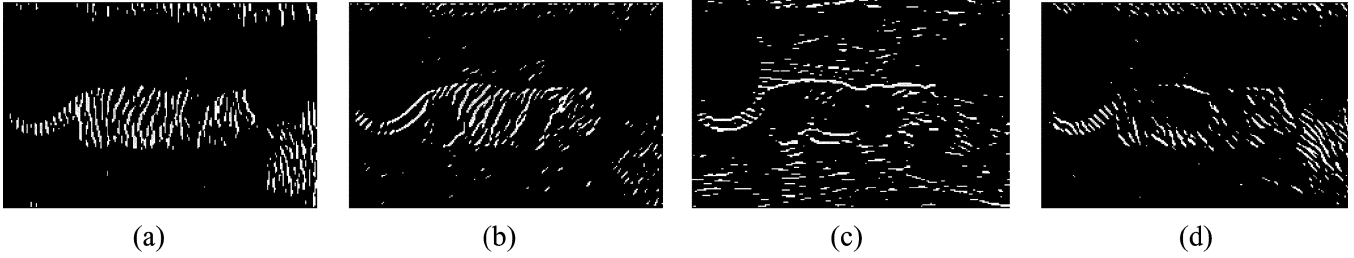
Fig. 8. Texture features extracted for the natural image depicted in Fig. 7(i) using Gabor filter with four orientations: (a) 0^\circ , (b) 45^\circ , (c) 90^\circ , and (d) 135^\circ .
